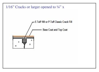
This detail describes the saw cutting of the 1/4" x  $\frac{1}{4}$ " saw cut being filled with the mixed water and P-Tuff Classic or E-Tuff 100. PTS fast cure Sealants E-101 or E-102 may be also used to fill the saw cut joint. All cracks 1/16" or larger must be saw cut to  $\frac{1}{4}$ " x  $\frac{1}{4}$ ".
