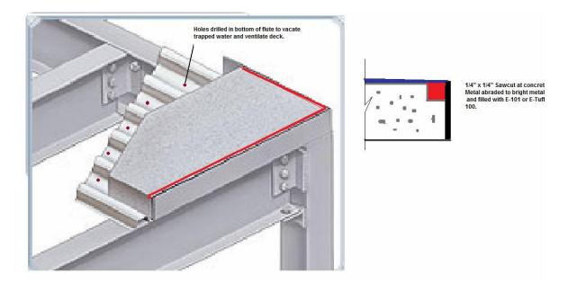
In the above detail,  $\frac{1}{4}$ " x  $\frac{1}{4}$ " minimum saw cut joint is formed at the metal edge where the concrete has separated from the metal edge support or T-Bar. The joint may be filled either with PTS-101 or PTS E-102 Joint Sealant.
