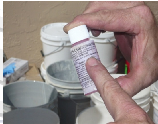
#8 Start by adding 1/2 vial of catalyst, use more to cure faster. Use more in low temperatures and less in high temperatures.
