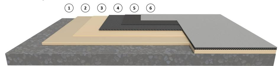
Concrete- It is preferred to have an ICRI profile of CSP 1. Surface can be profiled, cleaned, and prepared for CFRP application with TuffPrep cleaner. EnviroClean may be used for cleaning any dirt, grease, or oil build up.
