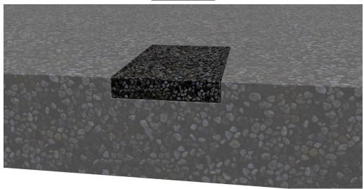
Fill blockout with PSI 3/8" polymer treated aggregate.
