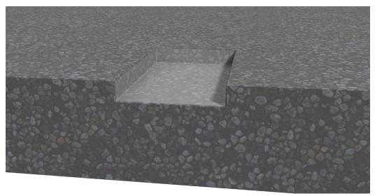
Saw cut concrete to prescribed width and depth. Remove concrete from blockout area. Prepare concrete subgrade by mechanical means to create a clean sound surface and apply TuffCrete Primer if required.
