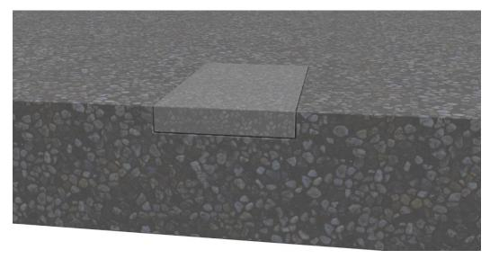
Pump TuffCrete MM into aggregate or hand place TuffCrete SP polymer into void. Finish with PSI Topping Sand and open to traffic when set.
