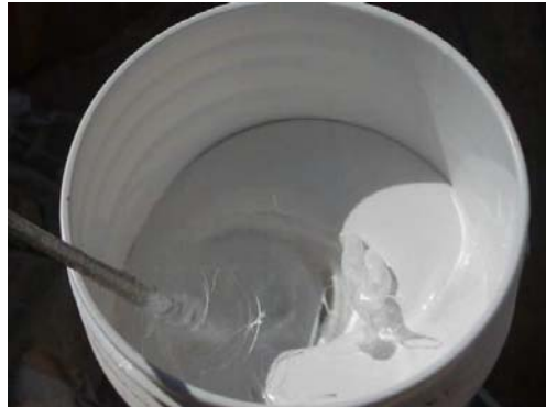
#8 Mix water and catalyst into the coating until the water completely disappears into the coating. Mix sides of pail leaving no water around the edges.
